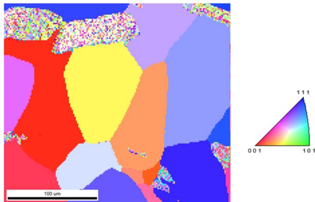
Figure 6: EBSD map for tantalum with small grains at discharge conditions of 5 mA, 1 kV using 0.41 ml/min argon flow after sputtering for 1.5 h. Corresponding inverse pole figure legend to the right.
