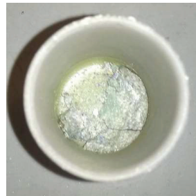
Figure 7: Crucible from experiment #13, 1700 °C and 1 l/min flow rate. The surface area of the metal is clearly reduced due to excessive evaporation.
