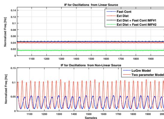
Fig. 6. Instantaneous frequencies (IF) for linear and non-linear sources of oscillations
