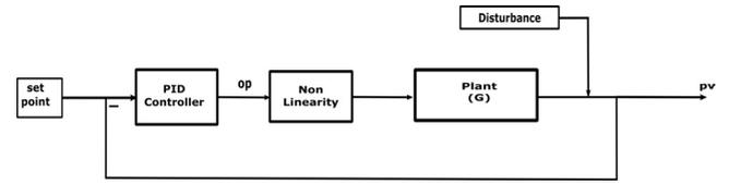
Fig. 3. Closed loop model
