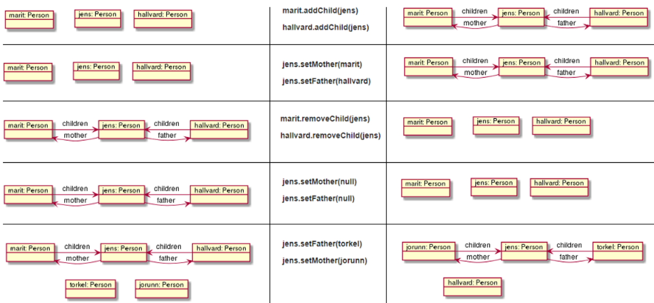
FIGURE 1 Graphical representation of the code-debugging task. The consistencies that were absent from the original version of the code. (1) Gender consistency: the mother should be a female and the father should be male. (2) Child-parent consistency: if Jens is the child of Merit, Merit should be the mother of Jens; and vice-versa. (3) The removal of a child-parent relationship from either a parent or a child should also apply to the whole family. (4) Adoption consistency: the child-parent (addition and removal) and the gender consistencies should be maintained in the case of an adoption
