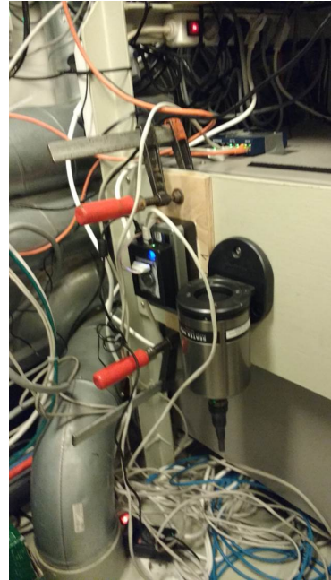
FIGURE 8. Alternative IMUs clamped to ship construction in the instrument room, close to the permanent MRU 5+ located in the same room. Photo: Astrid H. Brodtkorb, 2016.
