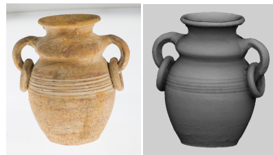
Figure 9: One (out of 31) synchronized image of a small vase obtained with the DI-One system (left) and the reconstructed 3D mesh (right).
