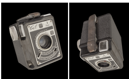
Figure 12: Views of a 3D model of the 1938 Durst Gil camera reconstructed from two shots taken at different object poses.
