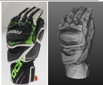
Figure 13: One (out of 93) image of a glove obtained by rotating the system basement around the Z axis (left) and the reconstructed 3D mesh through photogrammetric process (right).
