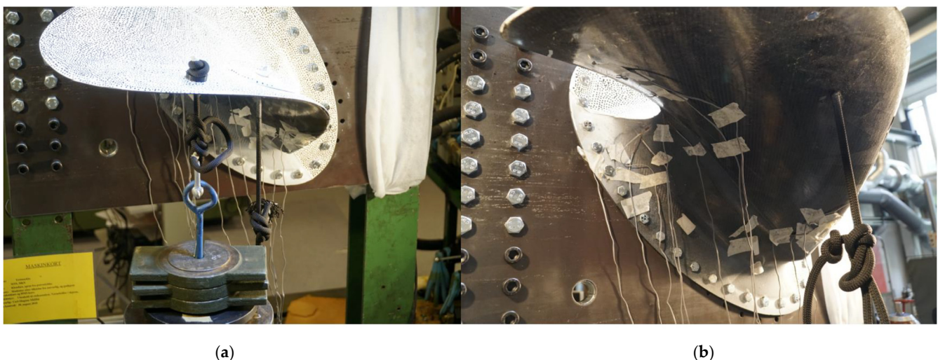
Figure 9. (a) The load was applied by hanging metal weights. The CFRP propeller blade is loaded with 500 kg, 375 kg at the 0.7 radius line and 125 kg at the 0.9 radius point in the left photo. (b) The strain gauges were attached on the blade and the root.
