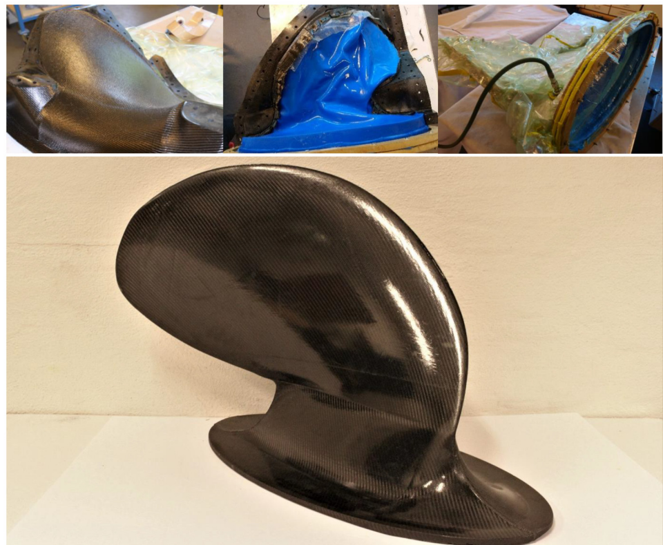
Figure 8. CFRP layup on a mould half, mould half with layup and silicone bladder, the assembled mould before oven curing cycle and the finished cast after demolding. Photos from [9].
