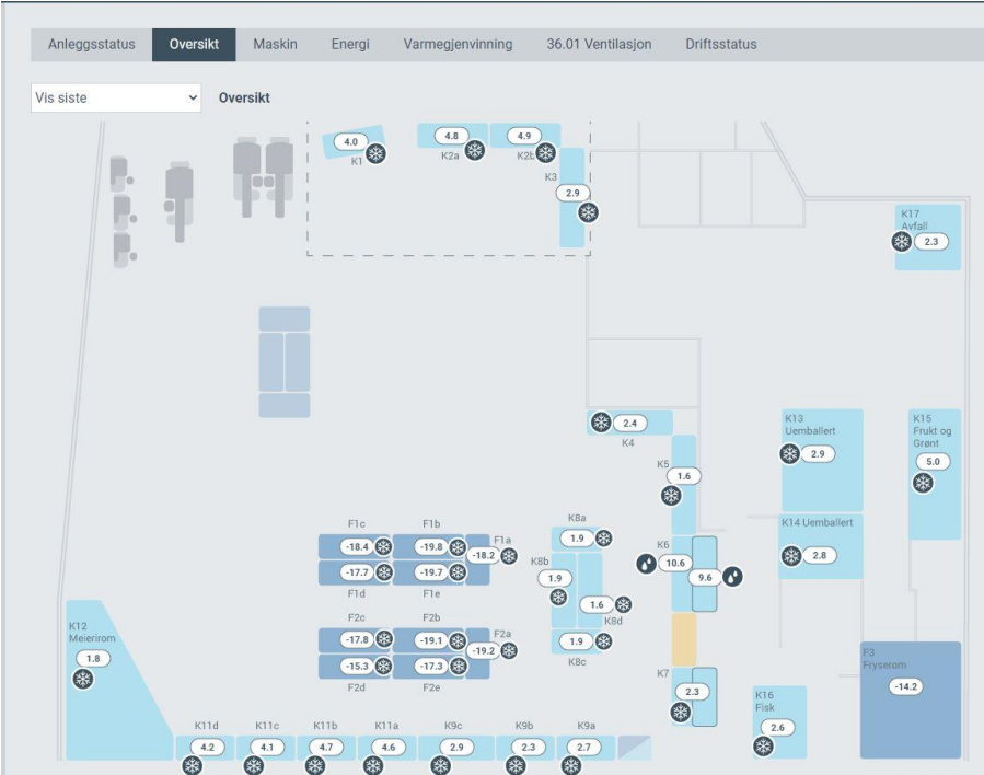
Figure 8-4: Screenshot IWMAC overview of the cabinets
