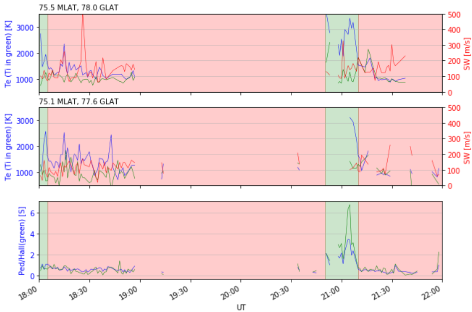
Figure 6.5: Timeseries of electron temperatures (blue), ion temperatures (green) and spectral widths (red) on the 8th of January 2012. The temperatures are measured by the ESR field aligned dish and the SWs are measured by the Hankasalmi radar. Green and red shading indicate close and open field lines respectively. Height integrated Hall (green) and Pedersen (blue) conductivities are also shown.
