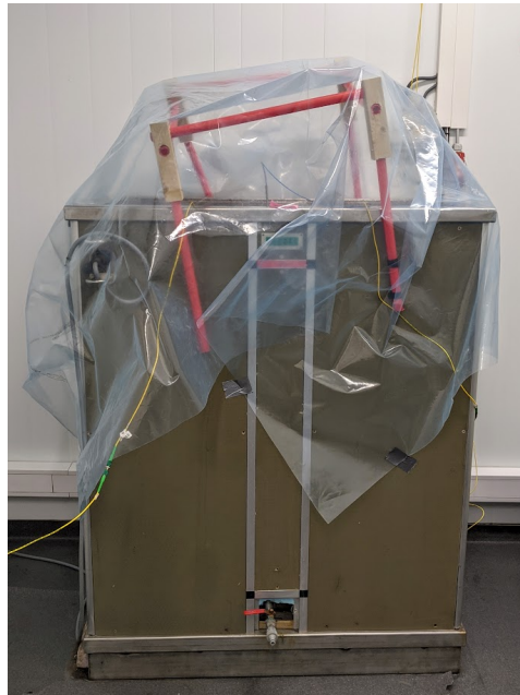
Figure 3.13: Plastic covering over ice tank to prevent evaporation.
