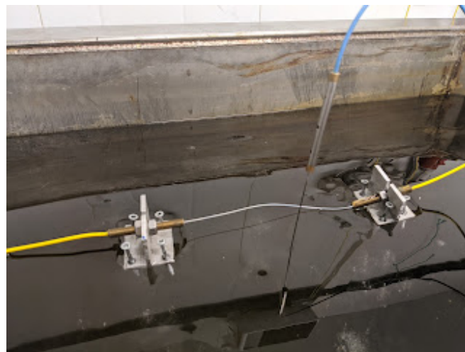
Figure 3.14: Displacement of sensors after 24 hours of installation. Sensors were reinstalled in an adjacent position on the ice every 24 hours of experimentation.
