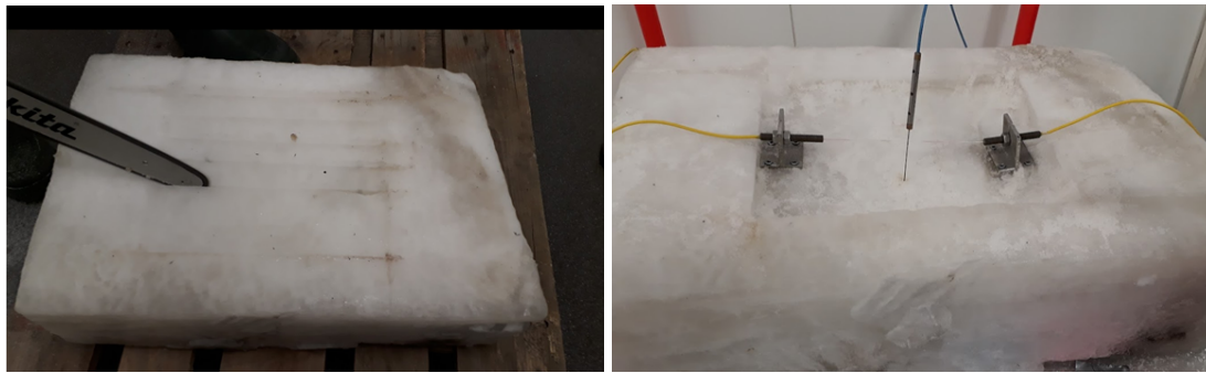
(a) Method for constructing pool in granular saline ice sample with chainsaw. (b) Empty pool in saline ice sample before seawater was added.
