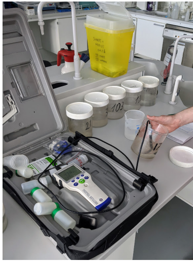
(a) Salinity measurement method.
