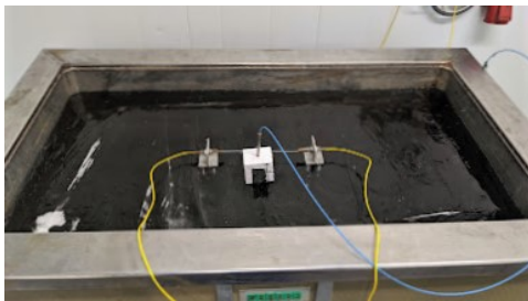
(a) Experimental lab setup with a strain and temperature sensors installed on the freshwater ice sample.
