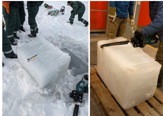
(a) Ice sample extraction process on Vallunden lagoon. (b) Sawing sample at UNIS before cold lab experiment.
