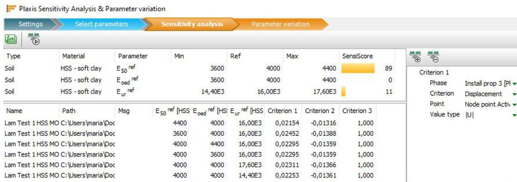
Figure 5.7: PLAXIS sensitivity analysis and parameter variation of the HSS model with scenario HSS01.
