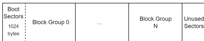
Figure 2.7: Typical Ext4 volume layout, adapted from Fairbanks [64]. The volume is composed of N block groups, starting from block group 0. If the block is greater than 1024 bytes, then the boot sector padding at the start of the volume is included in block group 0, where it is followed by the superblock and group descriptor table [62]
