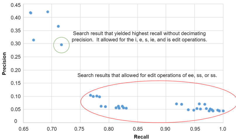
Figure 4.1: Summary of experimental results. Notation describes which edit operations are allowed in the approximate search: i for insertion, e for deletion, s for substitution, and pairs of letters denotes combinations of edit operations.
