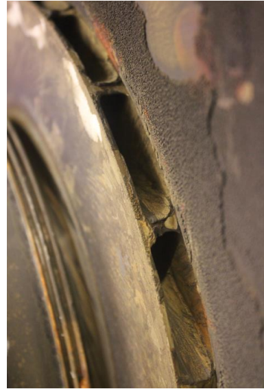
Figure 17 Wet gas compressor deliberately fouled during testing at K-Lab. The picture shows the impeller tip and the diffuser.
