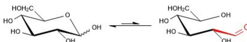
Figure 2.3: Depiction of the of the open and closed ring forms of a glucose reducing end saccharide, displaying the aldehyde functional group available for further reactions.
