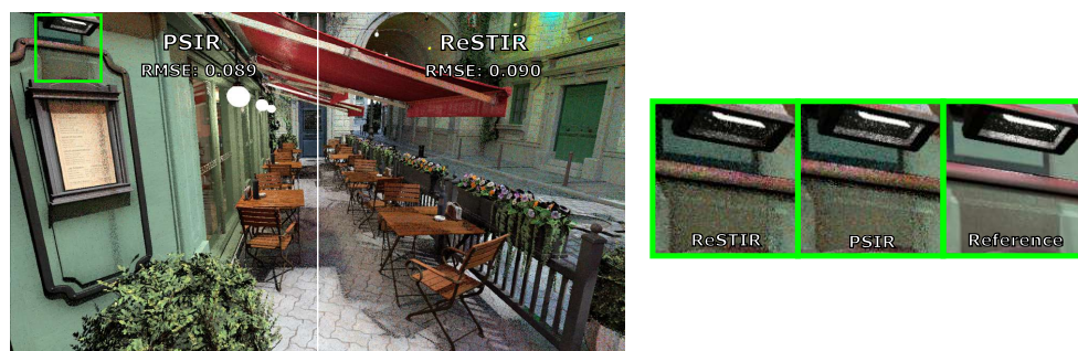
Figure 5.5: Snapshot of BISTRO (at day time) rendered with PSIR and ReSTIR, only using temporal resampling . There are only minor differences between ReSTIR and PSIR, both qualitatively and quantitatively.
