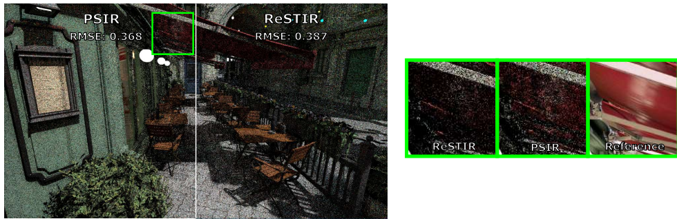
Figure 5.6: Snapshot of BISTRO (at day time) rendered with PSIR and ReSTIR, only using spatial resampling , from the same view as Figure 5.5 . There are visibly larger differences between PSIR and ReSTIR when temporal sample reusage is omitted.
