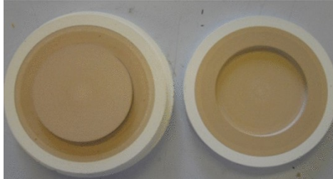
Figure 4: Example of a stepped index dielectric lens called a Luneberg lens. Each color change in this picture is a slightly changed ceramic. Several ceramic layers are poured and cast individually before assembling into the final lens. Reprinted from[17]
