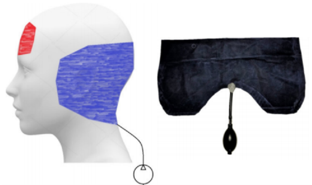
Figure 3.1: Pressure zones and design of one large inflatable element
