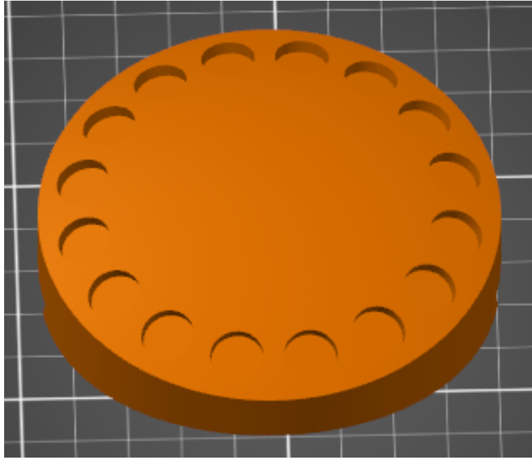
Figure 4.16: The helmet part of the magnetic connection seen from above. The holes are for the magnets.
