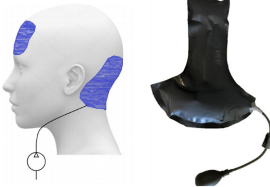
Figure 3.4: Pressure zones and design of the inflatable element with a forehead pillow
