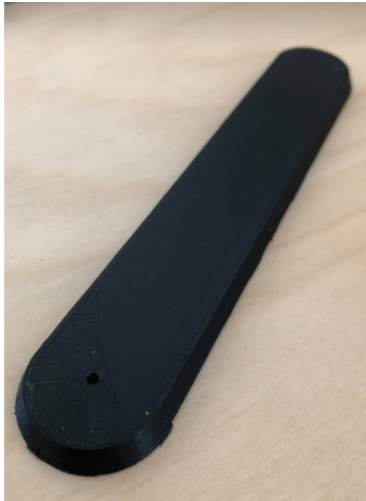
Figure 4.18: The wedge used to lock the helmet to the magnetic connection
