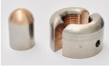
Fig 1. Electrical contacts made of W/Cu (80/20). Pin is the fixed contact (cathode) and split tulip is the dynamic one (anode).
