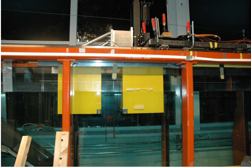
Figure 4.2: Picture of the experimental set-up without appendages. Here the model is located close to left beach. To change the hull to include appendages, only the gray profiles of the moonpool edges are exchanged with corresponding appendage profiles.
