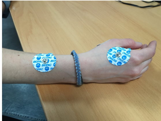
Figure 29: The placement of the electrodes.
