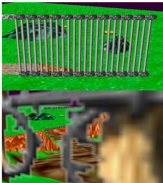
Figure 21: The first picture shows a transparent grid. The Second picture shows two transparent object without proper sorting.
