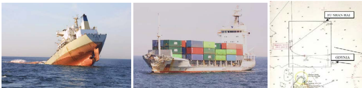
Fig.1: Left: ‘Fu Shan Hai’ sinking after the collision, Middle: ‘Gdynia’ after the collision. Right: Chart reconstructing the ship movements for the final 18 minutes up to the collision, DMA (2003)
