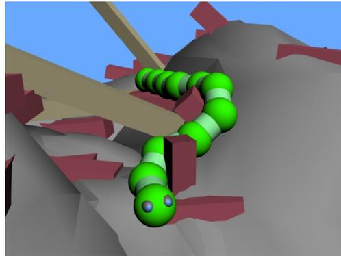
Fig. 1. Illustration of *obstacle-aided locomotion* with a snake robot.
