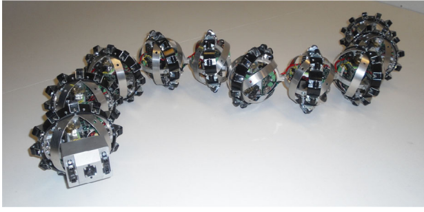
Fig. 6. The snake robot used in the experiment.
