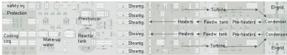
Figure 8-2 Identifying the main components in the IRD large screen display
