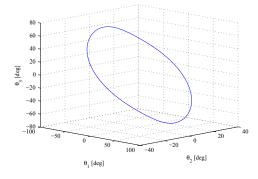
Fig. 10. The limit cycle traced out by the link angles of the snake robot.
