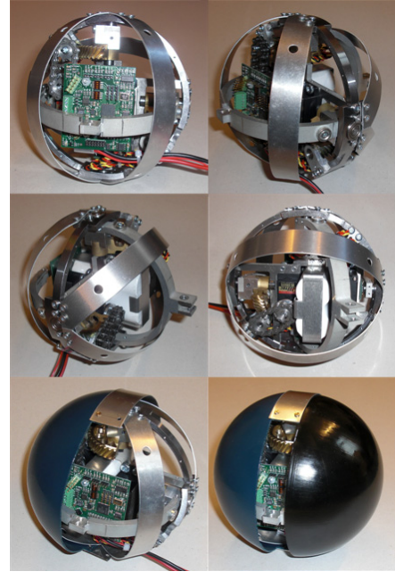
Fig. 6. Joint mechanism with spherical shell and support plates.
