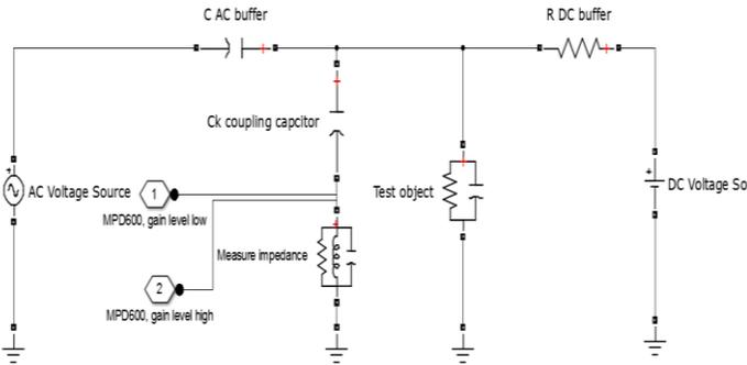
**Figure 5.** The test circuit – straight circuit with coupling capacitor.
