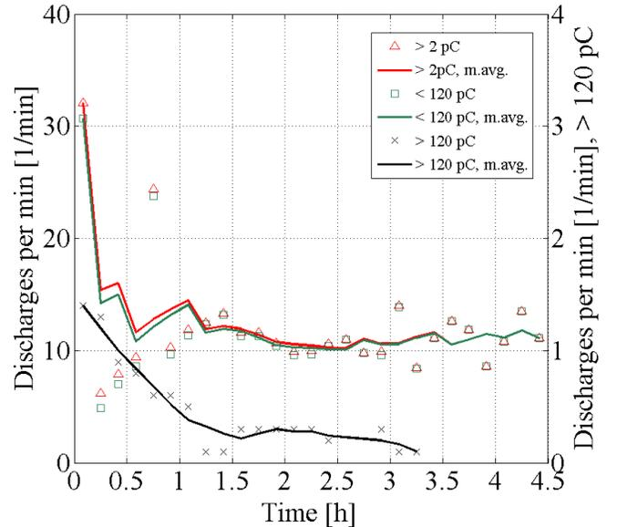
**Figure 6.** Discharge repetition rate for discharges for all, above and below 120 pC in test object at 10 kV DC,  $80^\circ\text{C}$ . Sampling interval is 10 min. The y-axis on the left give the repetition rate for discharges above 120 pC.
