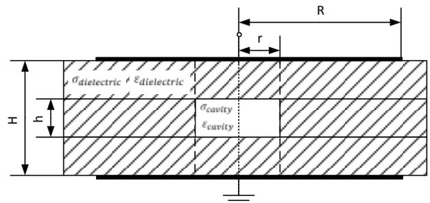
Figure 1. Structure of test object, three layer of films with cylindrical hole in the middle layer
