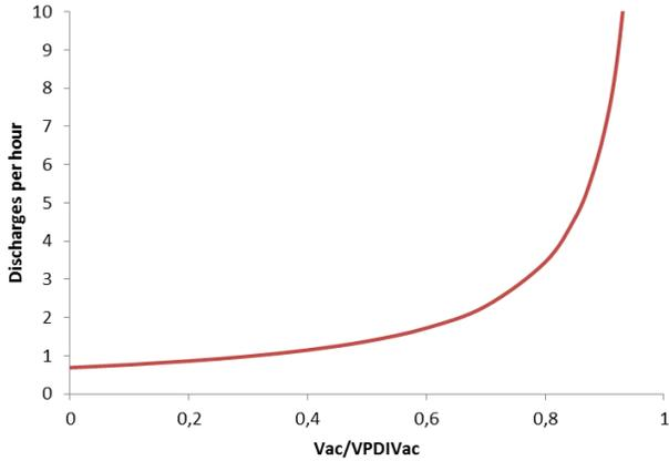
**Figure 4.** Discharge repetition rate as a function of ratio of AC voltage to AC partial discharge inception voltage, according to (13). The DC voltage is constant and above the DC partial discharge inception voltage.
