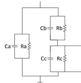
Figure 2. ABC equivalent circuit with RC-elements
