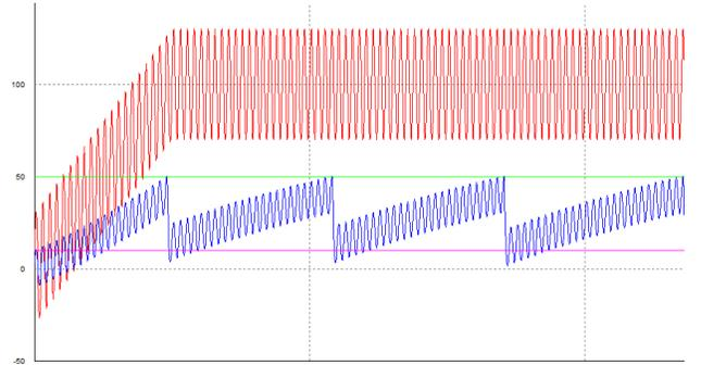
**Figure 3.** Breakdown of cavity voltage under combined AC and DC voltage, generalized plot. AC frequency lowered to better show the waveform. Red line: voltage over the test
