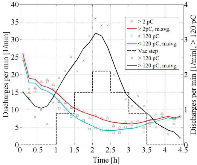
**Figure 7.** Discharge repetition rate for discharges for all, above and below 120 pC. 10 kV DC and 300, 500 and 700 V<sub>rms</sub>, at 80 °C. Sampling interval is 10 min. The y-axis on the left give the repetition rate for discharges above 120 pC.
