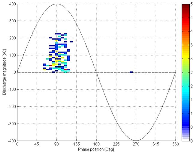
**Figure 8.** Discharge density plot versus phase angle of the AC voltage. Measured at 10 kV DC + 500 V<sub>rms</sub> AC, color bar shows number of discharges occurring during 20 minutes of applied voltage.
