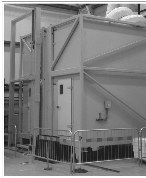
Figure 5. The large-scale guarded hot-box test facility used for the measurements.
