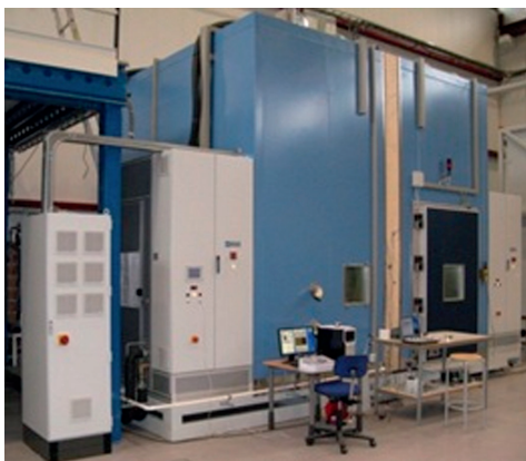
Fig. 3. The climate simulator used for the PCM-glazing measurements.
