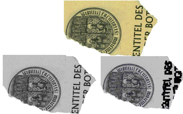
Figure 5.5: Top, an input image. Bottom left, corresponding grayscale output image with window size 10. Bottom right, another output image with window size 20. In output images, identified text zones are marked with black blocks.
