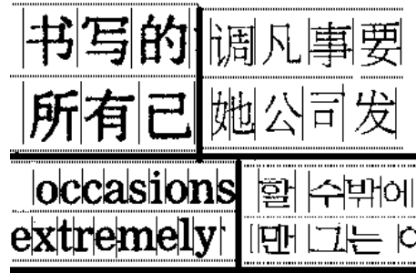
Figure 9.1: Line and Character segmentation results on Japanese (Top left), Roman (Bottom left), Chinese (Top right) and Korean (Bottom right) documents are shown.
