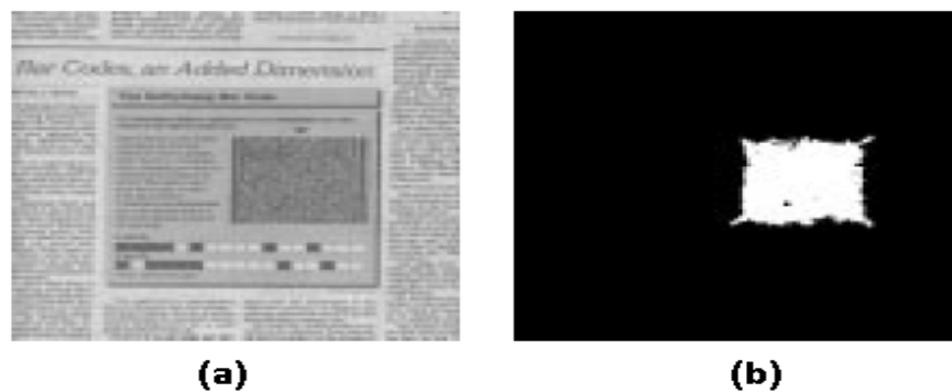
Figure 2.2: Locating bar code in a newspaper image. (a) A scanned image of a newspaper that contains a bar code. (b) The two-class segmentation using Gabor filter features. The bar code region in the image has a distinct texture.Figure adopted by author from [136]. Copyright with World Scientific Publishing Co.
