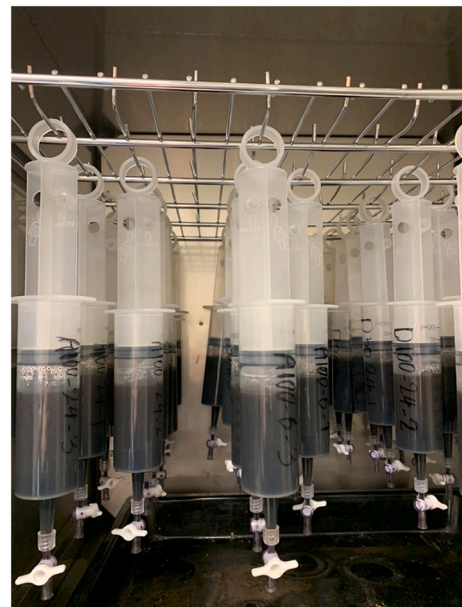
Fig. 1. 100 mL medical syringes have been used as batch anaerobic digester.
