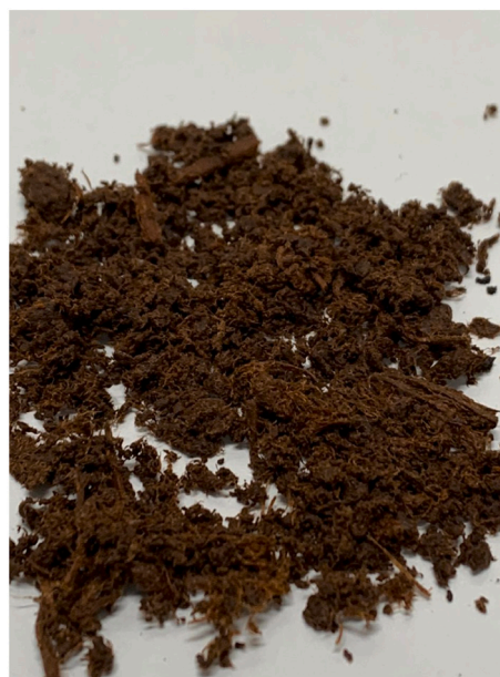
Fig. 2. SEBW. 30 mm birch wood chips were converted to a sticky, low fiber residue of dark brown color.
