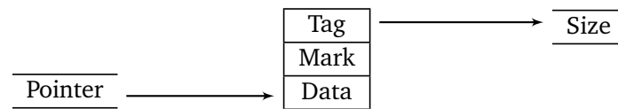
Figure 2.4: The structure of every allocated block on the Oberon system heap, based on a figure in [2].
