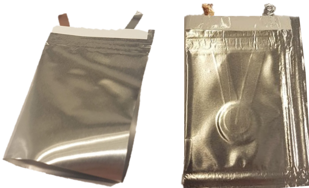
Figure 3.4: Left) Picture of pouch cell after the initial step, Right) Pouch cell when completed, being fully sealed with the active cell inside
