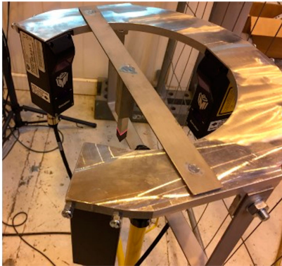
Figure 10. Rope shape scanners with calibration piece. This figure is available in colour online.
