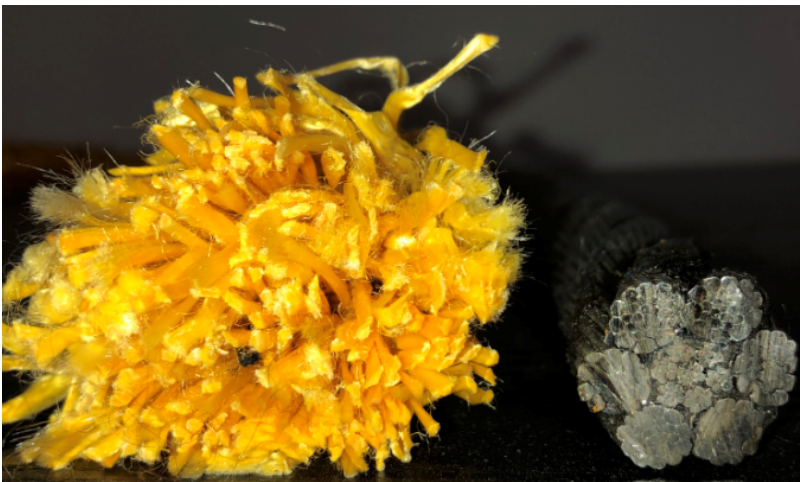
Figure 1.7: Subcomponents of fibre rope compared to steel wire rope
