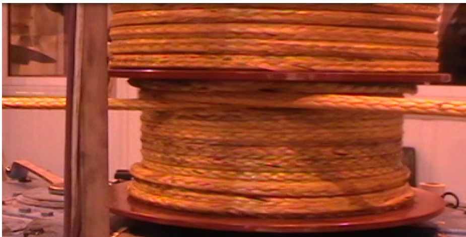
Figure 4.40: Rope stuck in the underlying layer during rope on rope friction test
