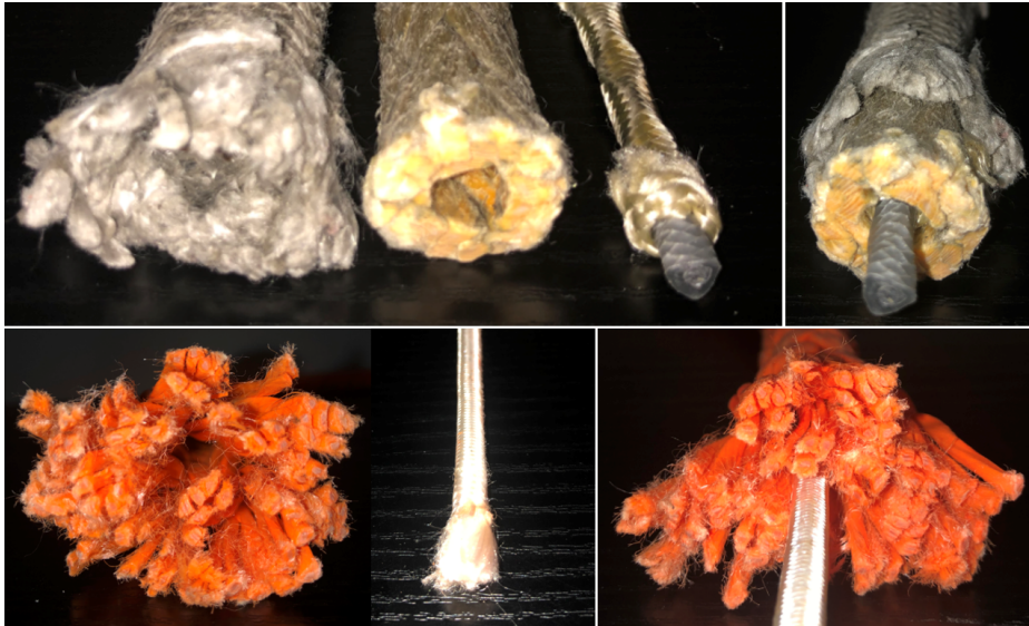
Figure 2.3: 12-strand braided ropes with shape stabilizing measures
