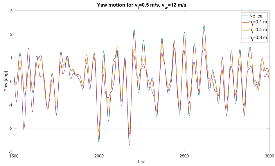
Figure 5.41: Yaw motion time series for v_i = 0.5 m/s, v_w = 12 m/s and different ice thickness
