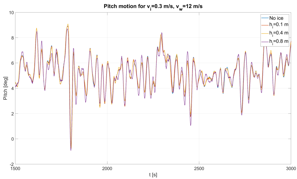
Figure 5.36: Pitch motion time series for v_i = 0.3 m/s, v_w = 12 m/s and different ice thickness
