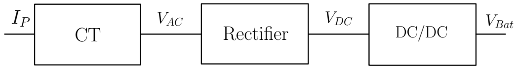
Figure 1.3: A block diagram of the magnetic energy harvesting system that contains a CT, a rectifier and a DC/DC converter.
