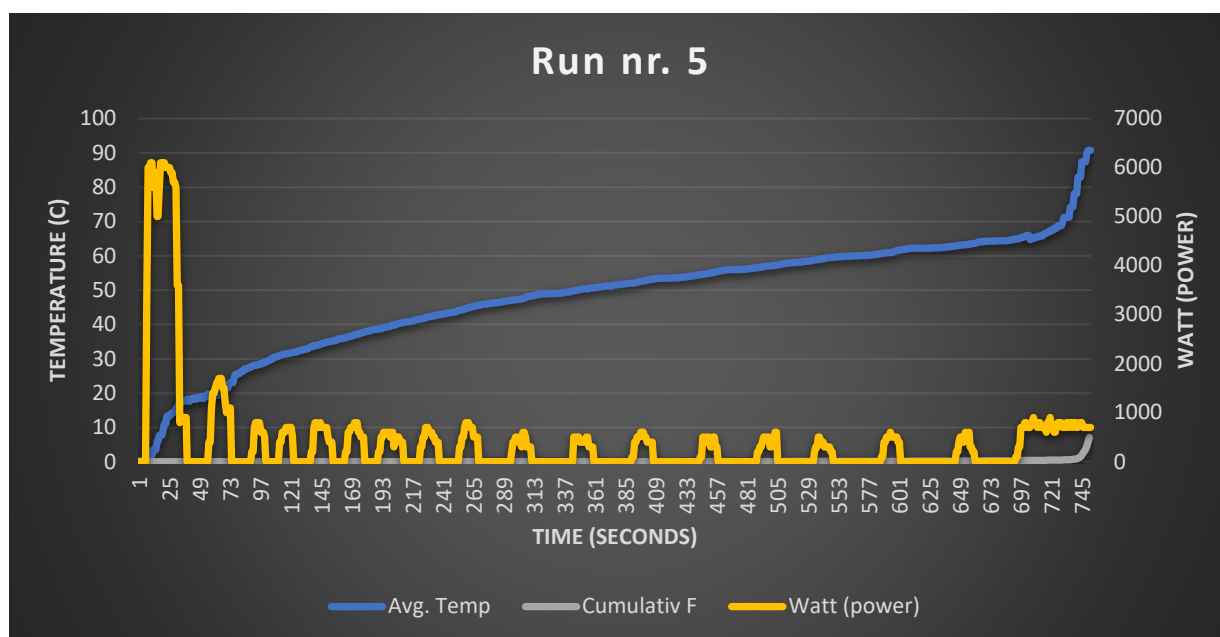
Figure 5. Illustrates the temperature increase for the cold spot of MW run nr.5: Total energy absorbed during the whole treatment was 323.4 kJ, F-value was a total of 0.0021 min. The yellow plot shows the cycles of Watt introduced to the cauliflower.
