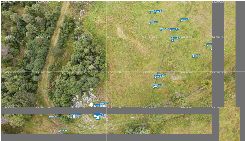
(b) Tiled 4K-image. Note that the model made predictions on each tile individually. This image was stitched together after the test was run.
