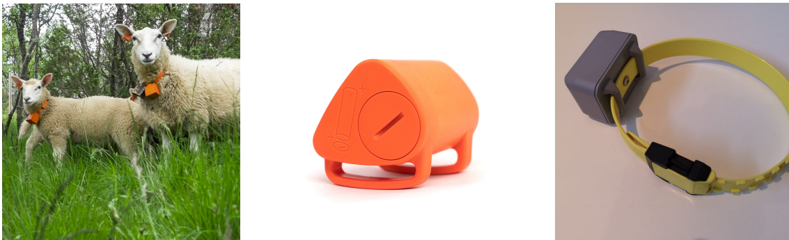
Figure 2: Example of radio bells. Findmy [9], Telespor [10] and Smartbjella [11] respectively.
