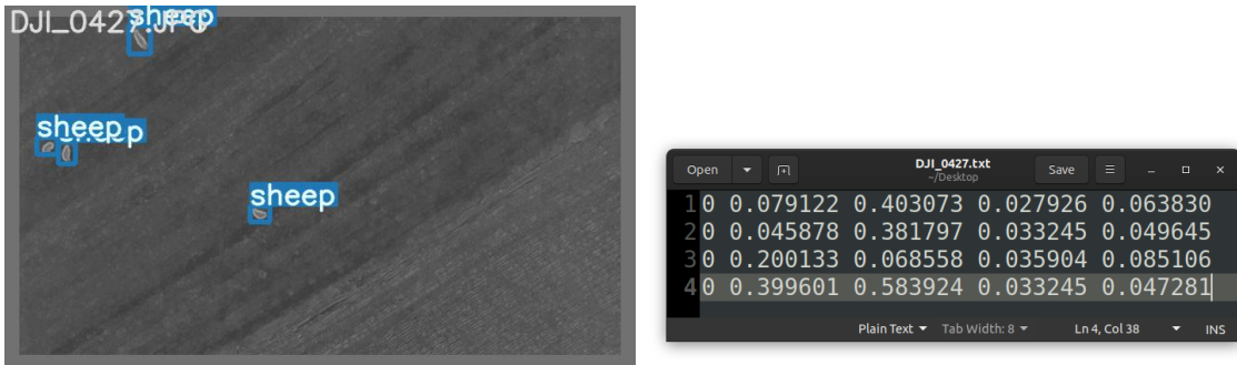
Figure 9: An example image with its labels displayed, and the corresponding text label file on YOLO-format.
