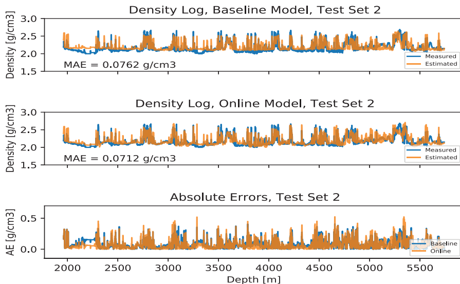
Figure 3.6: Measured and estimates on test set 2. Top: Baseline model performance. Middle: Streaming learning performance. Bottom: Absolute errors (AE).
