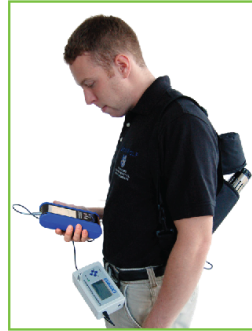
FM-801 (on included ACC-BELTCL-1 belt clip) shown connected to GrayWolf AdvancedSense Pro
