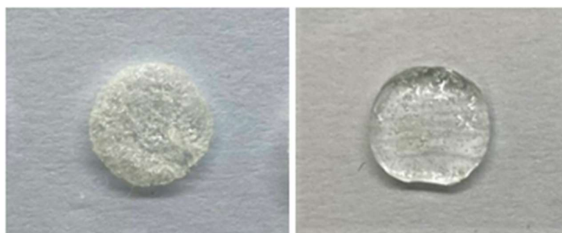
Figure 20: Appearance of the foam scaffold used in this study. To the left is a dry alginate foam as they come delivered from NovaMatrix®, taken out of the 96-well plate. To the right, a foam supplemented with 10 µL 3DLife buffer for demonstration of foam appearance after absorption of liquid.
