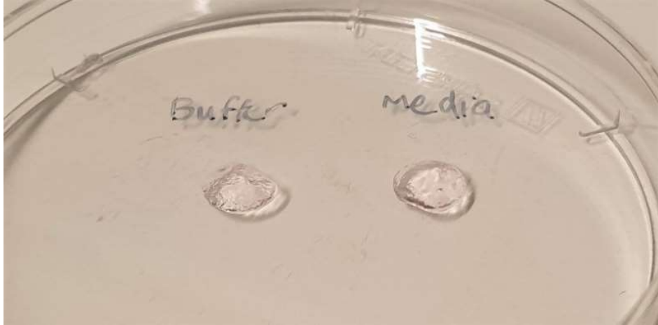
Figure F1: Qualitative comparison of alginate foam gelled with 1% (w/v) alginate in buffer (left) and 1% (w/v) alginate in cultivation media (right) after 48 h. No differences were found.
