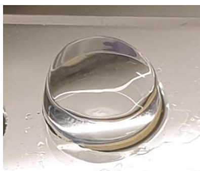
Figure 21: Appearance of the hydrogel scaffold used in this study. This 1% alginate gel (65 \mu\text{L} ) was casted in removable rubber wells on a glass plate for testing gelation, without cells.
