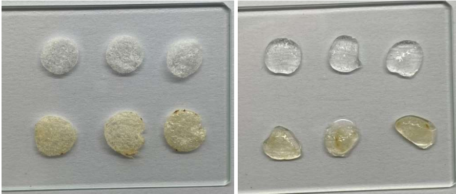
Figure F5: Alginate foams from the first batch used (top row) and later batch (bottom row) taken out of the 96-well plate. Dry foams are shown in the left image, and foams added buffer are shown to the right.
