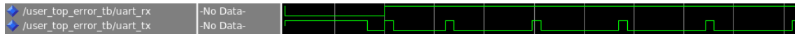
Figure 4.9: Holding the RX line low causes a stop bit error, which triggers the transfer of a frame with the according flag (orange). The stop bit flag can be observed in the second bit of the first byte. Note the reversed bit order.
