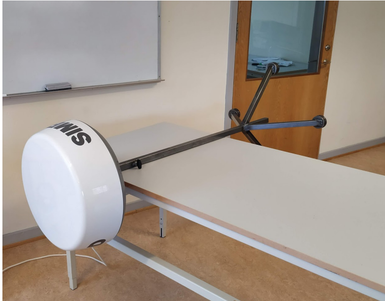
Figure 2.6: Image showing the radar being put on its side to avoid fading due to the rotating antenna.
