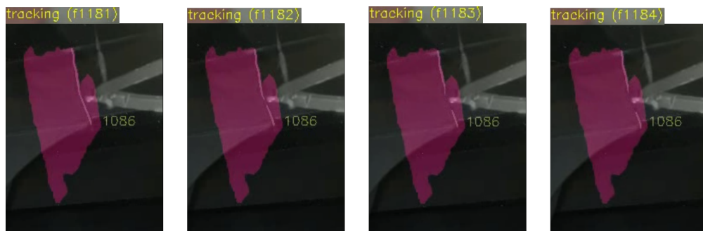
Figure B.7.: Frame 1181 to 1183 in "A_tracking.mp4". A crack can still be tracked through occlusions. The white line is the detected crack, while the red area is the track. The base video depicts a none-planar scene, therefore the inaccuracies in the track are so noticeable.
