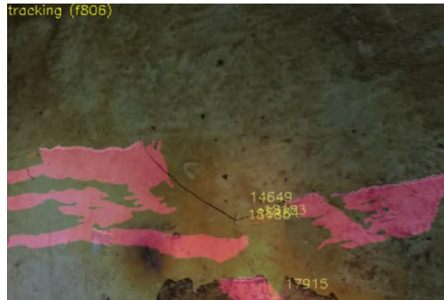
Figure B.6.: The tracks of the same frame as in B.5. Inaccuracies in the MC also accumulate in the tracks
