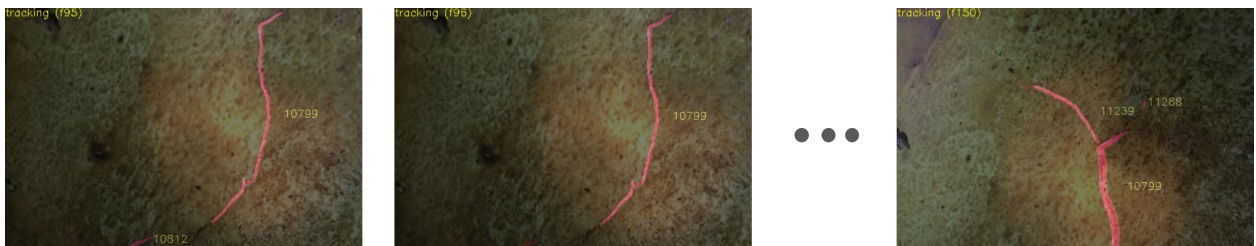
Figure 4.19.: The output of the tracking module on video "C" at frame 95, 96 and 150. The crack instance ID 10799, stays consistent
