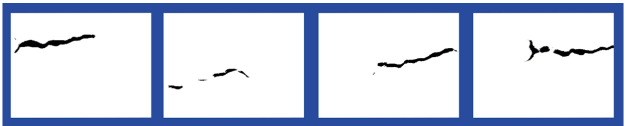
Figure 3.3.: An example of the predicted label maps outputted by an arbitrary crack detector. The detector is run over a 4 frame video sequence, from right to left, making the label map most to the left the most recent. Each black pixel corresponds to a crack in the input frame. Note that there is some camera movement between the frames and that this detector is inconsistent with its prediction
