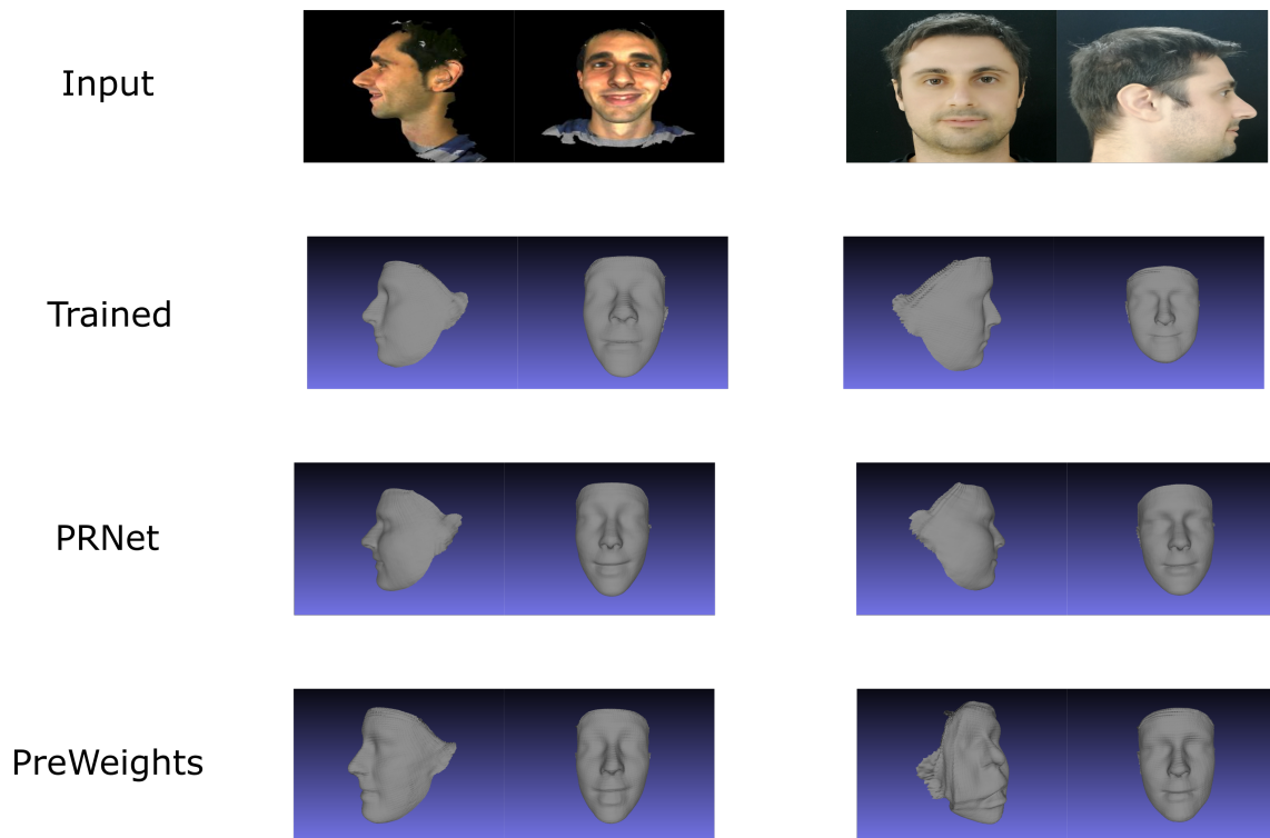
Figure 5.2: Reconstruction results from different models. "Trained" is the proposed method trained as described in 4.2, "PreWeights" is the proposed method using only the weights from [2]. Image to the left is from MICC Florence while the one on the right is from a proprietary Norwegian University of Science and Technology dataset.
