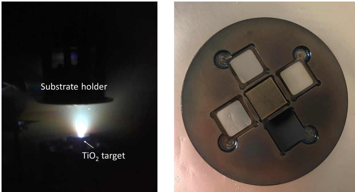
Figure 4.1. The left picture is inside the PLD chamber during the plume deposition, substrate holder, and TiO 2 target. The right image is the substrate holder, and it is four-hole for substrates.
