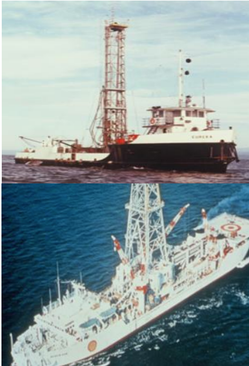
Figure 4: Eureka DP equipped vessel (top) and SEDECO 445 first DP rig (bottom) (26)
