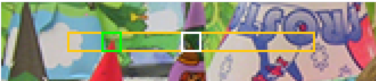
(b) Initial search position (white box) and true match (green box) in the right image. The yellow box shows the horizontal search line.
