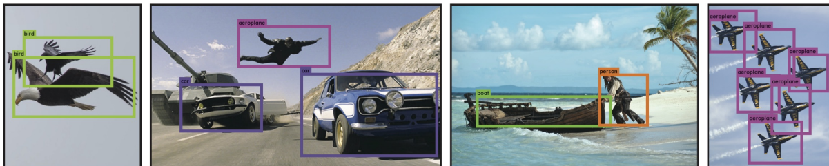
Figure 3.2: Example result from object detection. The outputs are bounding boxes and class predictions for each object of interest in the image. Image courtesy by Redmon et al. (2016).
