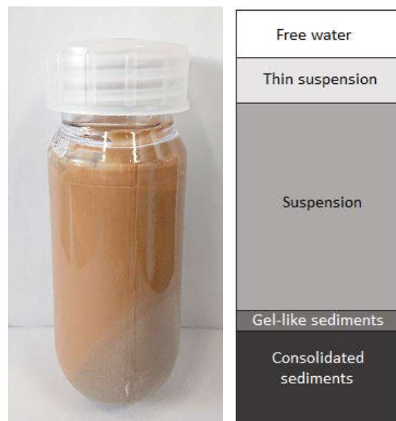
Figure 1. Bentonite/barite fluid sample after centrifugation and a schematic illustration of the sediment layers.
