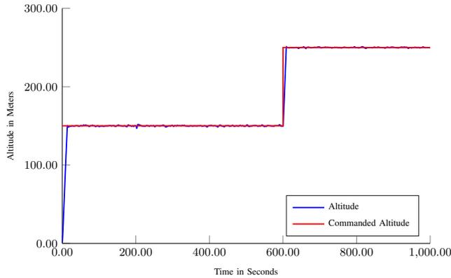
Fig. 2: Commanded and resulting altitude of the UAV
