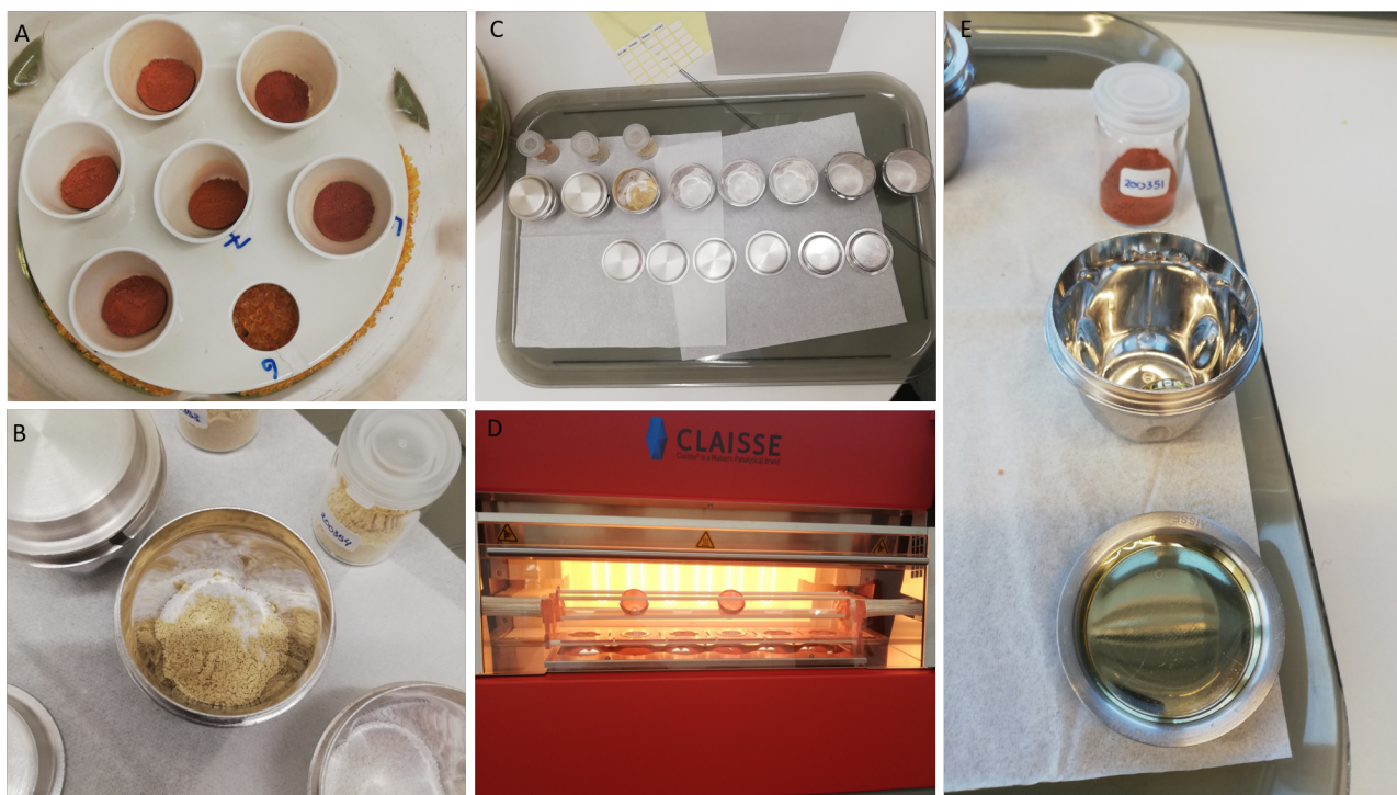
Figure 4.5: The preparation for main element analysis by XRF. A) Samples after ignition, B) & C) Powder mixed with the flux-agent in platinum crucibles, D) The TheoX advanced fluxer furnace from Claisse, E) Solidified glass pill in platinum container.
