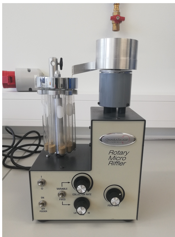
Figure 4.8: Quantachrome micro riffler used to split the sediment samples in order to make polished blocks.
