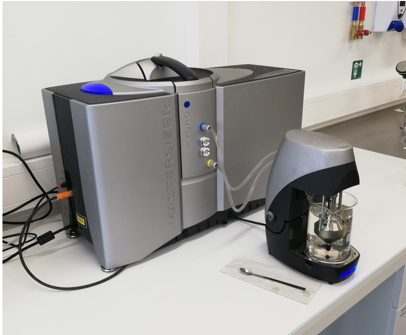
Figure 4.7: The set-up for particle size determination showing the malvern Mastersizer 3000 with the HYDRO EV disperser in the front
